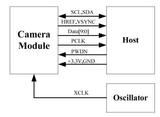
The host may have integrate camera interface like STM32F2 or STM32F4 series MCUs, or ARM9/11 which has dedicate camera port, and DPS like TI TMS320DM series, as well as FPGAs that user can design special logic for camera application. The typical connection between these
