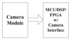
For the host that doesn't have a dedicate camera interface, additional hardware is needed. User need to buffer a entire frame before read them out with low speed MCUs. For example <u>ArduCAM shield</u> is a additional hardware that can be connected to Arduino UNO/Mega board, user can take a photo or something like that easily. The following diagram show the system without dedicate camera interface.
