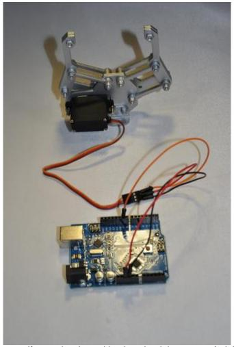
One of the quickest ways to see if your claw is working is to hook it up to an Arduino. I used an Uno, but any 5V Arduino compatible board can be used to control the claw. The three colored wires from the servo are as follows:
