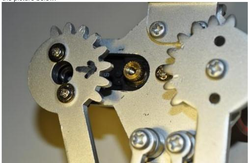
Make sure and turn the servo gear counter clockwise until it stops and make sure the claw is clamped and in the "closed" position. The reason for this is because the servo only goes 180 degrees. If you do not put it in its max counter clockwise position, the claw may not open all the way, or at all.
